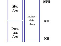
Remember that if you use a 256 byte derivative it is possible to get an "Out of Data Space" error from the linker even when you have used only 80H bytes of **data**. You still have access to the rest of memory (80H - 0FFH), but you must specify **idata** for variables that can be located in this range.
